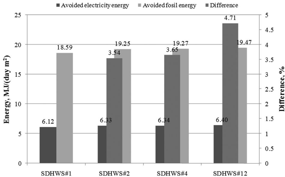
FIG. 12. Maximum annual amounts of avoided electricity, and avoided fossil energy for different SCs for Belgrade. Also, the difference of these variables compared to the stationary solar collector is given.
