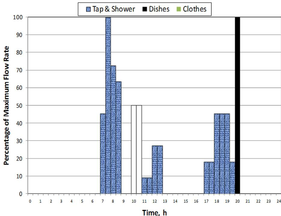
FIG. 3. Schedule of DHW use for (a) tap and shower (0.0000945 m<sup>3</sup>/s maximum with 43.3 °C) (b) dish and clothes washer (0.000063 m<sup>3</sup>/s maximum with 50 °C). Dish-washer operates daily, while cloth washer on Sundays.
